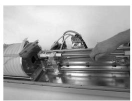
Remove the piston rod from the linear slide using 5 mm hex key
