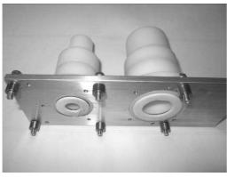
Pull the spacer rings on the screws and screw the front plate back to place.
