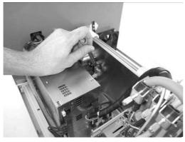
Loosen the safety nut with 10 mm wrench.
