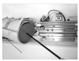
Pull out the piston and remove the old O-ring seal. Before replacing it clear the inside surface of the cylinder and the groove on the piston from old lubricant and dirt.
