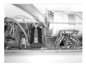
Unscrew the fixing rod from the cylinder's back end.
