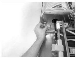
Disconnect the temperature sensor on the cylinders back end.
