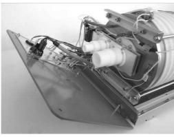
Carefully fold down the main front panel, taking care of the cables connected to it.
