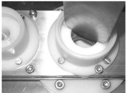
Remove the pneumatic outlets.
