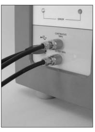
• The lower BNC connector [Gated 1 MHz] is an output with the gated 1 MHz.
