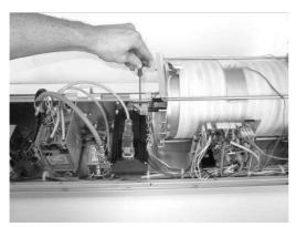
Loosen the grub screw on the fixing element with 3 mm hex key.
