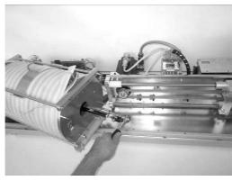
Unscrew the 4 nuts on the tightening screws with 13 mm wrench and remove the cylinder's back end.
