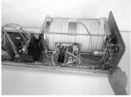
Use 10 mm wrench to loosen the nuts on both side.
