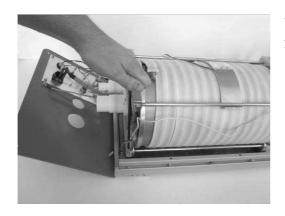
Unscrew the 4 screws on the cylinder's feet with 5 mm hex key.
