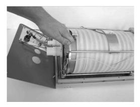
After replacing the piston, put the back cylinder plate in place and loosely screw the nuts on the tightening screws.
