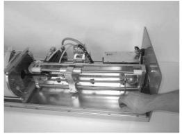
Loosen the 4 screws fixing the rear bearing block with 4mm hex key.
