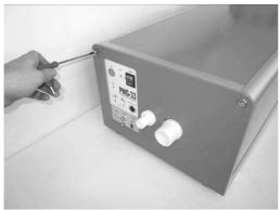
Unscrew the 4 screws with 4mm hex key.
