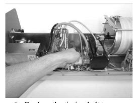
Move the piston by hand until the fastening plate coincides with the mounting hole
