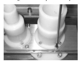
Unscrew the 6 screws with 4mm hex key. Carefully pull off the front plate of the BTPS valve.
