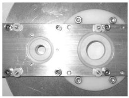
The rollers with their shafts should be put back in place if they fall off.
