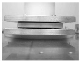
The slider plate should be in middle position.
