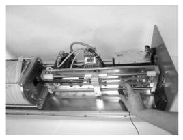
Plunk the lower part of the belt to generate sound. You can use a universal belt tension meter or a simple PC microphone and chromatic FFT tuner software to measure the frequency.
