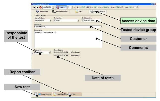
History of entered data is automatically stored, and [Manufacturer], [Device type], [Customer] and [Tested by] fields have auto complete feature.
