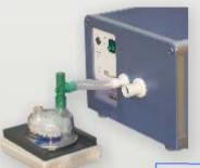
PWG-33BT provides full BTPS simulation for all types of exhaled curves
